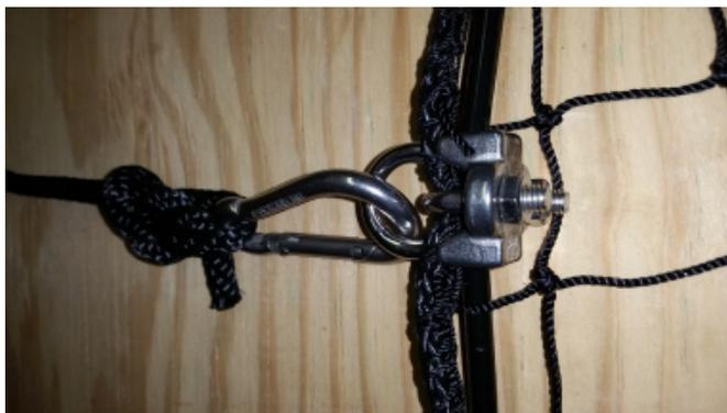
**Photo 4A** (Clip, O-ring, Cable Clamp Assembly attached to Pull Rope & Clip)
