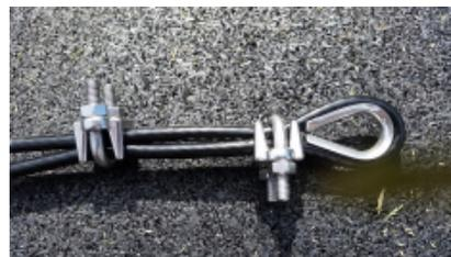
**Photo 3A & 3B** (Turnbuckle and Cable Clamp Packs / proper install method)
